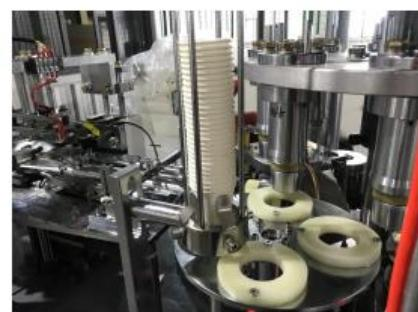
3. Aluminum disc indexing adopts **open cam**, maintenance and lubrication is more convenient and simple than gear box divider, the space of transmission parts in the machine is large, and it is easy to operate and maintain. It is superior to similar products on the market in all aspects, and can replace similar models on the market.
